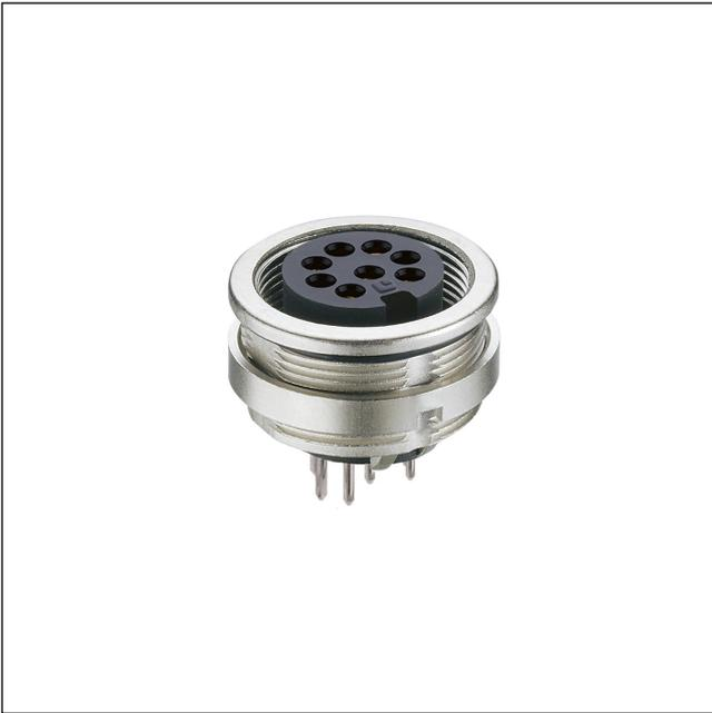
SWUM™ chassis socket acc. to IEC 61076-2-106 and AISG specification, IP68/67, with threaded joint, for printed circuit boards, manual soldering, for front mounting
